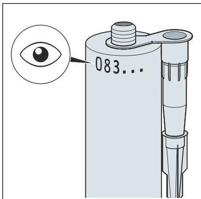
Fig. 13: Filling date of the mounting adhesive
