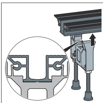
Insert the drain socket
