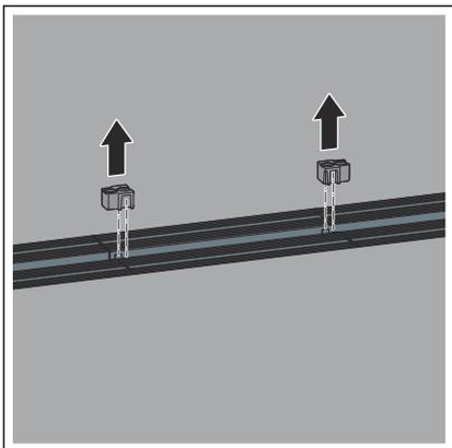
► Remove the spacers when using extension pieces.
