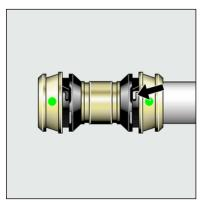
Check the insertion depth in the inspection window.
