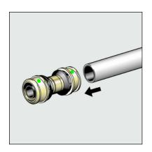
Push the pipe into the press connector until the pipe end is visible in the inspection window.
