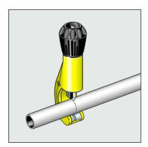
Cut the pipe to length using a pipe cutter (model 2191).
