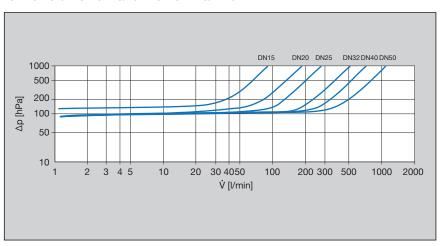
Fig. 2: Performance diagram pressure loss CRV press/threaded connection
