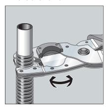
Cut the protective pipe to length using the protective pipe cutter (model 5341).
