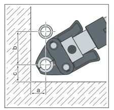
Space requirement Picco, Pressgun Picco, Pressgun Picco 6, Pressgun Picco 6 Plus
