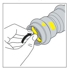
Insert a new, undamaged sealing element into the bead.
