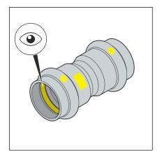
Ensure that the complete sealing element is in the bead.
