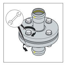
The simultaneous use of several tightening tools is possible.
