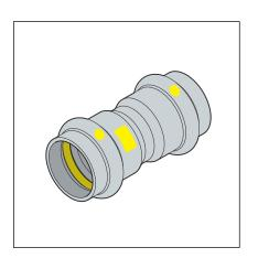
The press connectors have a circumferential bead in which the sealing element lies. The press connector is deformed upstream and downstream of the bead and permanently connected to the pipe during pressing. The sealing element is not deformed during pressing.
