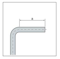
Pipes in the sizes d15, 18, 22 and 28 can be bent cold with commercially available bending equipment (radius at least  $3.5 \times d$ ).
