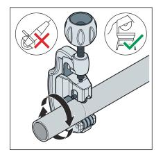
Cut the pipe at a right angle as accurately as possible using a pipe cutter or a fine-toothed hacksaw to ensure a complete and even pipe insertion depth.
