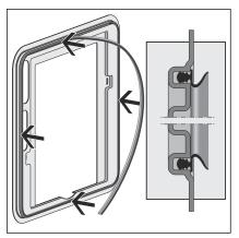
Fit the supplied seal in the cover frame on the front.
