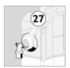
Screw the ½ inch connector into the wall lead-in.
