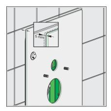
Check clearance between wall and cover plate (min. 5 mm).
