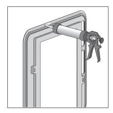
Apply the silicone seal to the rear of the cover frame.
