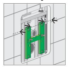
Mount the bearing surface (H support) for the cover plate flush with the finished wall surface (size 17 / 19).
