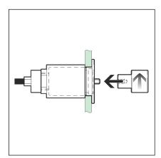
Screw the actuating button hand-tight onto the hydraulic cylinder from the front.
