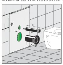
Adapt the length of the flushing pipe and drainpipe.
