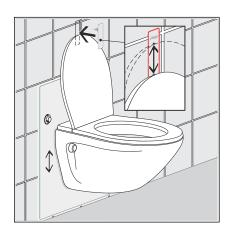
Depending on the version of the WC lid, it may be that there is contact with the wall during the height adjustment of the WC. Attaching the protective sticker prevents damage to the surface in the possible contact area on the wall and on the WC lid.
