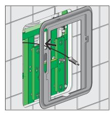
Lead hydraulic actuation unit through the cover frame towards the front
