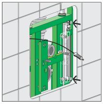
Insert new gas pressure spring and attach with Allen screws.
