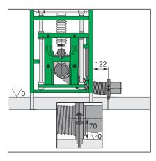
Alternatively: Secure the drain elbow onto the wall or floor without the fixing material supplied, taking into account the fixing sizes.
