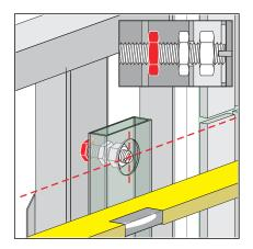
■ Tighten the rear threaded nuts at all four points of the H support (size 17).
