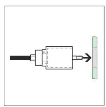
Insert the hydraulic cylinder from the rear through the opening in the cover plate.
