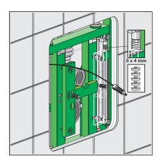
Place the relevant number of spacer washers below the piston rod of the gas pressure spring.
