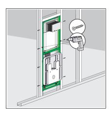
Screw the WC element together laterally with the support profiles (size 17).
