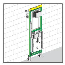
Attach WC element to the floor using the fork spanner (size 13) and the screws and dowels supplied.
