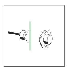
$\hfill \hfill \supset$  The actuating button has been mounted.
