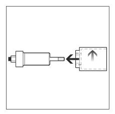
Screw the sleeve onto the hydraulic cylinder as far as it will go.
