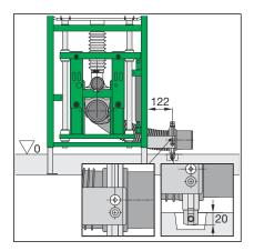
Attach drain elbow laterally onto the element using the fixing elbow supplied.
