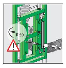
■ The radius of the hydraulic actuation must be at least 50 mm. This prevents the hydraulic actuation from buckling.
