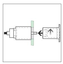
Screw the rosette through the cover plate from the front onto the hydraulic cylinder.
