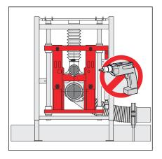
Plaster board must **not** be attached to the height-adjustable internal frame.
