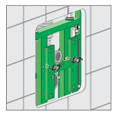
Unscrew the threaded rods for the fixing of the sanitary object to the required size.
