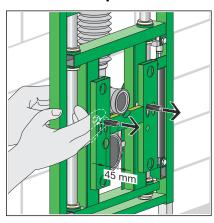
Unscrew the threaded rod of the WC fastening so that it projects out by approx. 45 mm.
