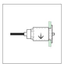
Counter screw the sleeve from the rear side.
