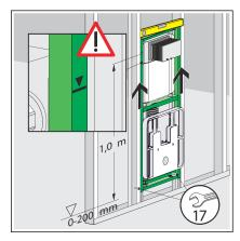
Determine construction height in accordance with the on-site marking of the upper edge of the finished floor.
