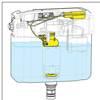
**Fig. 4: The motor operates the Bowden cable**
