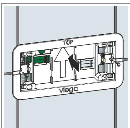
► Insert the base plate and secure with the supplied screws.
