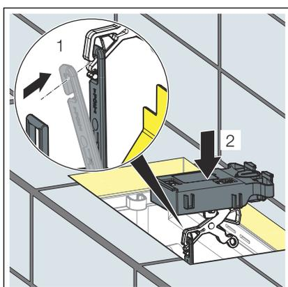
➤ Insert the mechanism.
