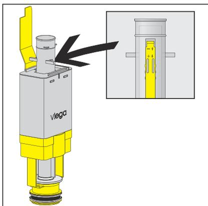
➤ Set the small flush volume at the slide control at the side of the overflow pipe.
