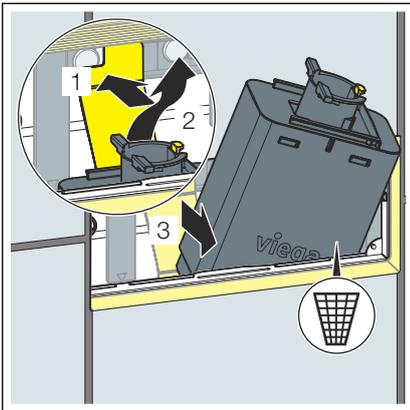
➤ Remove the drain valve and dispose of it.
