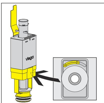
➤ Set the large flow volume at the slide control at the bottom of the drain valve.
