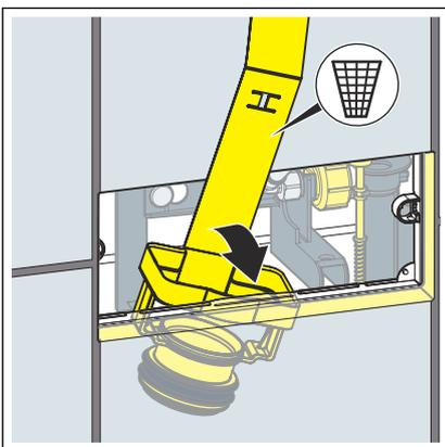
➤ Loosen the flap of the drain valve seat.
