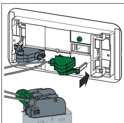
► Insert the Bowden cables into the back of the base plate.
