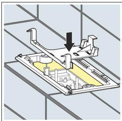
► Insert the support in the base plate.
