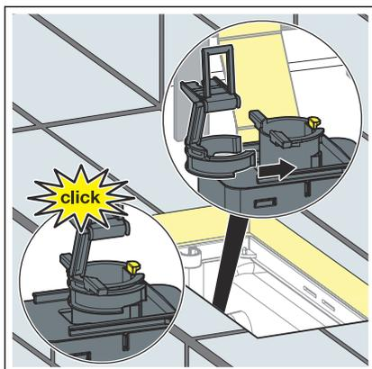
➤ Push the bow onto the drain valve from the left.
