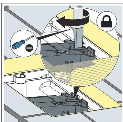
➤ Turn the mechanism's lock by 90° in a clockwise direction.
