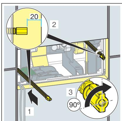
► Insert the enclosed threaded bolts into the drill holes inside the revision shaft and fasten them by turning them 90°.
