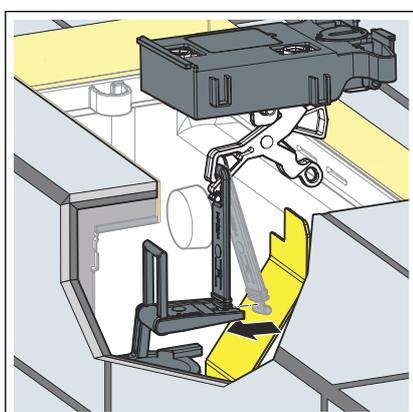
➤ Hang the bow of the drain valve in the clip of the mechanism.
