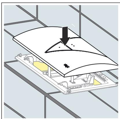
► Hang the flush plate from above in the base plate press in below.
