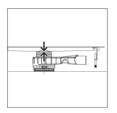
Check whether the shower channel is inserted into the height adjustment piece as far as it will go.
