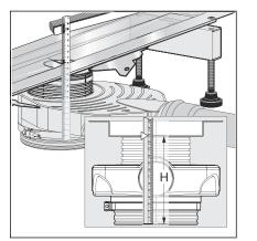
Determine the required height (see fig., dimension H).
