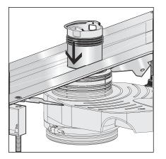
Measure dimension X from the upper edge of the immersion pipe and cut (X= H-Y):
