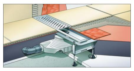
Fig. 2: Diagram of a bonded seal
