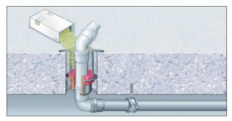
Fig. 4: Example: fire protection pipe lead-in
