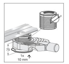
Push the floor piece in by one ring (1 x 10 mm). The fine tuning within these dimensions takes place using the height adjustment piece.
