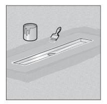
Apply the second layer of bonded sealing generously onto the sealing tape and floor screed.
