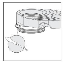
Loosen fastening ring with screwdriver.
