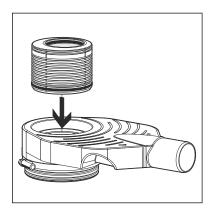
Insert height adjustment piece with O-ring.
