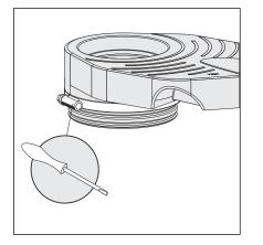
Loosen fastening ring with screwdriver.
