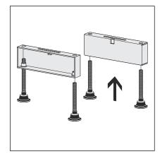
Screw the height adjustment into the foot.
