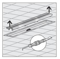
Remove grate, e. g.4965.90 with removal tool model , art. no. 689 704.
