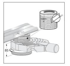
Shorten height adjustment piece accordingly. The water seal level remains 50 mm.
