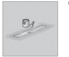
Apply the first layer of bonded sealing generously onto the screed. Observe the instructions for use of the manufacturer of the bonded sealing.
