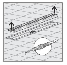
Remove grate, e. g.4965.90 with removal tool model, art. no. 689 704.
