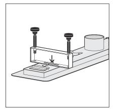
Push feet into the retaining brackets.
