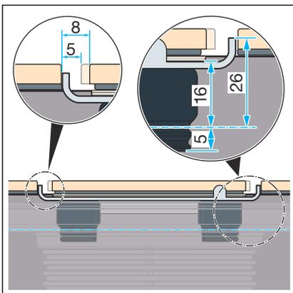
**INFO!** Drainage capacity with 5 mm inlet gap 0.4 l/s. Drainage capacity with 8 mm inlet gap 0.5 l/s.
