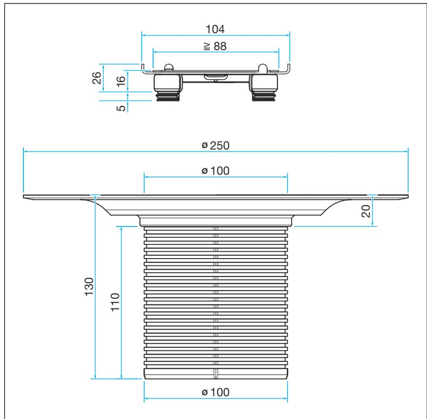
Fig. 2: Installation dimensions
