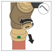
Screw in the extraction valve with a fork spanner (SW 17).
