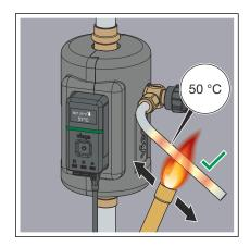
Heat the tube evenly. If the outlet pipe is heated evenly and the flame is guided carefully, there is no danger of damaging the valve.
