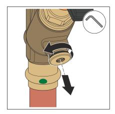
Unscrew the drain plug with an Allen key (SW 5).
