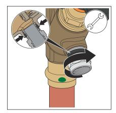
Screw in the adapter nipple with a fork spanner (SW 19).INFO! Screw in the Teflon® seal as far as it will go.
