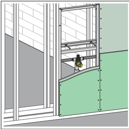
► Double-clad element (2 x 12.5 mm).
