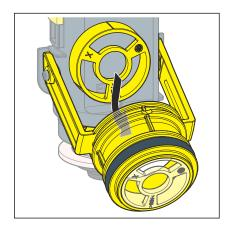
Insert the flushing throttle.
