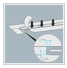
Press the sealing tape strips firmly onto the mounting adhesive and bonded sealing.
