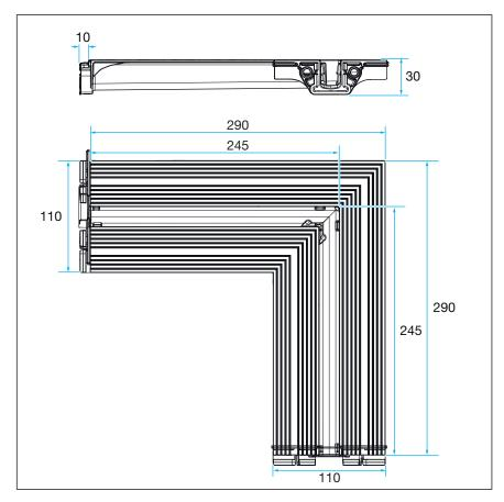
Fig. 17: Dimensions of connection piece  $90^{\circ}$
