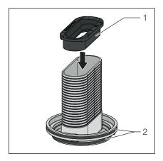
Mount the seal (1) and both sealing elements (2).
