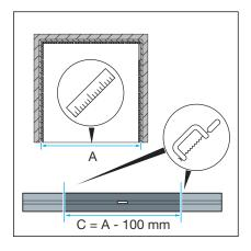
■ Calculate the profile length, also see ♥ Chapter 3.2.1 'Calculating the profile length in niche installation' on page 26.
