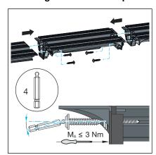
Screw the connector straight onto the profile.
