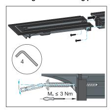
Screw the end closing piece straight onto the profile.
