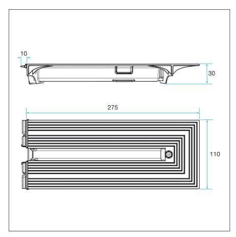
Fig. 16: Dimensions of end closing piece
