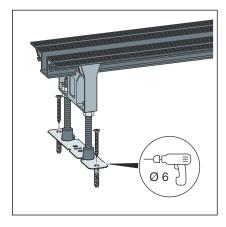
Secure the feet in place with the fixing material if required.
