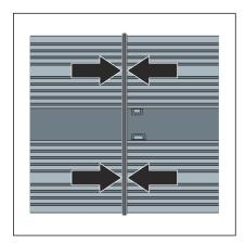
□ The connector is properly mounted when the seal is slightly pushed together.
