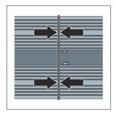
☐ The end closing piece is properly mounted when the seal is **slightly** pushed together.
