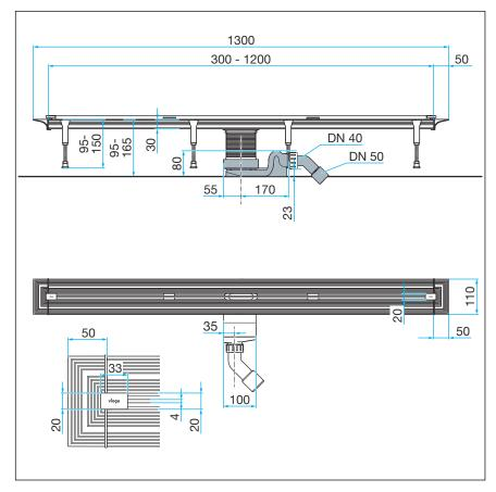
Fig. 14: Dimensions of base unit basic model
