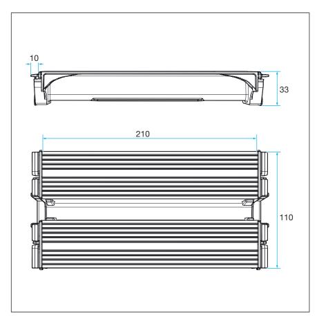
Fig. 15: Dimensions of connection piece
