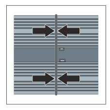
□ The 90° connector is properly mounted when the seal is slightly pushed together.
