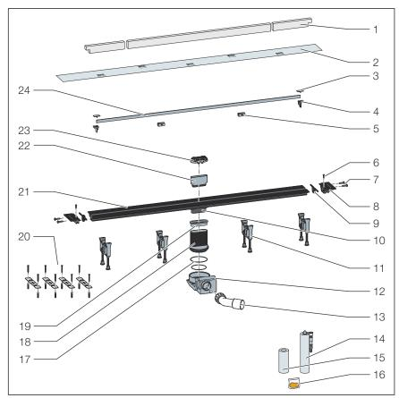
Fig. 6: Components and scope of delivery
