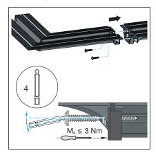
■ Screw the connection piece 90° onto the profile straight.
