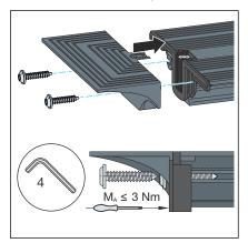
Screw the closing cap straight onto the profile.
