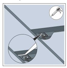
Connect the tile edge onto the channel side with tile adhesive or joint filler.
