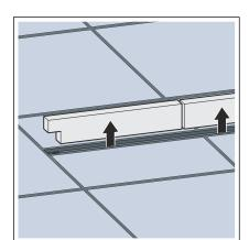
Optionally, a sieve can be inserted. When the sieve is used, the drainage capacity decreases by 0.05 l/s per drain.
