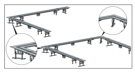
Fig. 20: When the  $90^{\circ}$  connector is used, an additional foot must be mounted below the corner angle.
