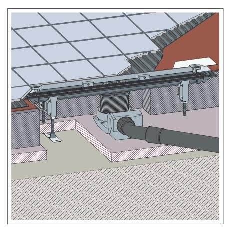
Fig. 10: Diagram of a bonded seal
