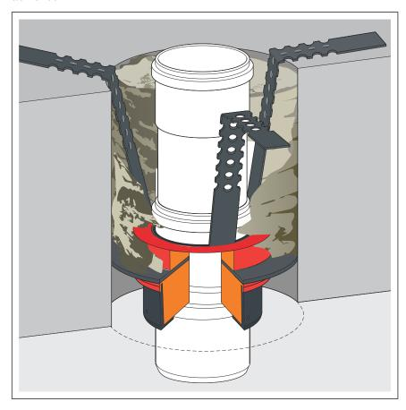
Fig. 12: Example: fire protection pipe lead-in
