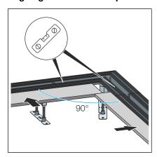
Align the shower channel and the 90° connector both horizontally and at a 90° angle to one another.
