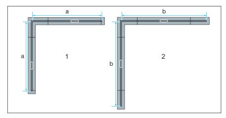
Fig. 4: Installation possibilities with connection pieces 90° for L version
