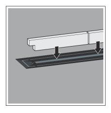
■ Cut the protective insert to size and insert.
