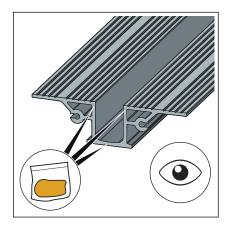
The profile must be lubricated with the enclosed grease in the area around the seal.
