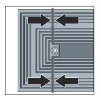
□ The closing cap is properly mounted when the seal is slightly pushed together.
