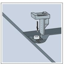
Place the standing grate holder on the screw and adjust it to the tile height.
