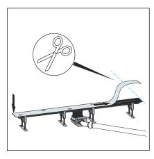
If necessary, shorten the protective foil and stick onto the flange.
