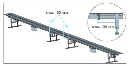
Fig. 19: Distance between fixing point and foot = max. 100 mm
