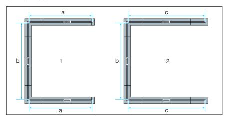
Fig. 5: Installation possibilities with connection pieces 90° for U version
