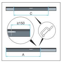
Transfer the length of the profile onto the shower channel.
