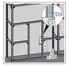
Set the height of the fitting holder according to the information of the sanitary item manufacturer.
