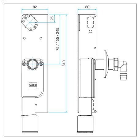
Fig. 2: Installation dimensions
