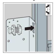
Use the slot nuts supplied to attach the fitting holder to the open mounting rail.
