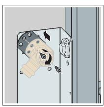
Attach the wall plate fixings and the wall plate.
