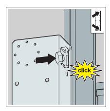
Push the slot nut in until it engages.
