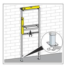
Attach element to the floor using the fork spanner (size 13) and the screws and dowels supplied.
