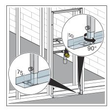
If necessary, adjust the pre-mounted foot depth from 75 mm to 50 mm: Pull out foot and turn by 90°.
