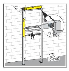
Set the installation depth of the element with the fork spanner (size 17).
