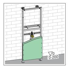
Double-clad element (2 x 12.5 mm).
