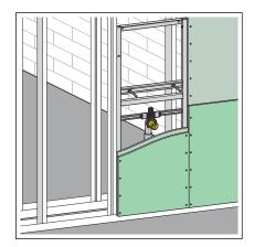
Double-clad element (2 x 12.5 mm).
