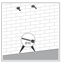
Remove WC element and drill floor holes.
