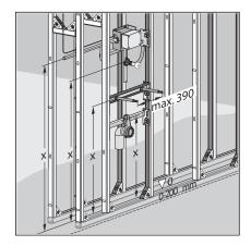
If necessary, align the height of the urinal element.
