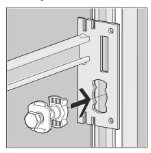
Secure the module onto the open side of the Steptec rail with the slot nuts supplied.
