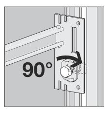
Press the slot nut in gently and secure in the open rail side with a 90° turn.
