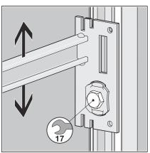
Tighten slot nut with a fork spanner (SW 17).
