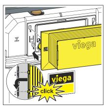
■ Place the inspection shaft on the site protection panel.
