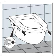
Loosen (do not remove) the fixing screws with fork spanner.
