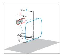
Flush actuation takes place without contact via an infrared sensor on the flush plate. This sensor differentiates between a close and a far range.
