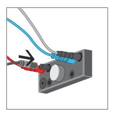
Connect the cable from the programming contact onto the control.
