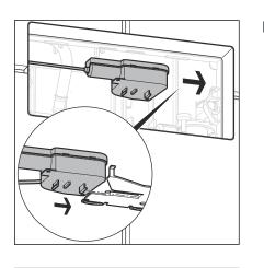
Push the drive unit onto the holding panel.
