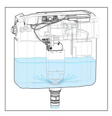
Fig. 5: The water flows into WC via the open drain valve
