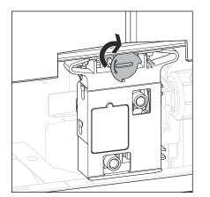
Turn the mechanism's lock by 90° in a clockwise direction.
