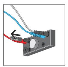
Remove the protective cap of the programming connection from the control.
