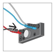
Connect the cable from the programming contact onto the control.
