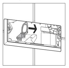
Push the holder for the battery compartment onto the spacer from the left.
