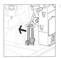
Press the bow backwards from the mounting of the mechanism.
