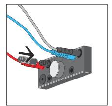
Place a protective cap onto the contact.
