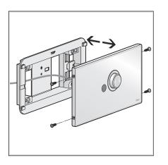
Remove the installation frame from the flush plate. Carefully lead the installation frame along the connection cable.
