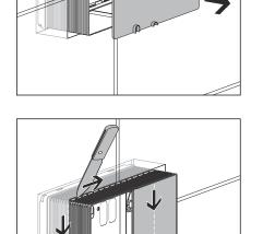
Score the revision shaft along the edge of the tiles with a knife. Angle the knife to do this so that the cut is made flush to the surface of the wall.
