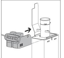
Push the Bowden cable unit onto the drain valve from the left. The Bowden cable unit must be felt to click into place on the drain valve.
