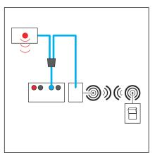
Fig. 8: Connection of radio controlled actuation
