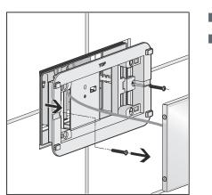
Loosen and remove the screws from the installation frame.
