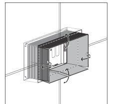
Bend out and pull down the sides of the revision shaft. The edge of the revisions shaft must be flush with the wall surface.
