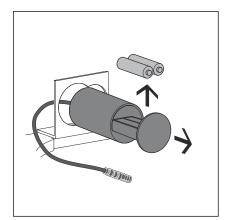
Open battery compartment and remove flat battery.
