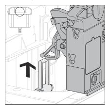
Hang the mechanism in the bow of the drain valve.
