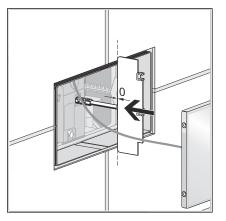
Set the length of the actuating rod with the template supplied. The tip of the rod must lie 2 mm behind the basic panel.
