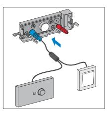
Fig. 2: Actuation of the flush via an external sensor
