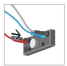
Place a protective cap onto the contact.
