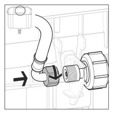
Connect the flexible hose to the filling valve.
