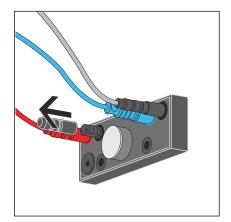
Remove the protective cap of the programming connection from the control.
