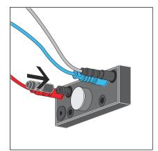
Place a protective cap onto the contact.
