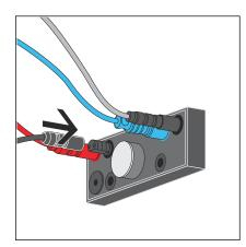
Connect the cable of the programming contact to the control.
