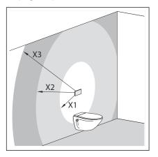
Fig. 9: Installation position of the power pack
