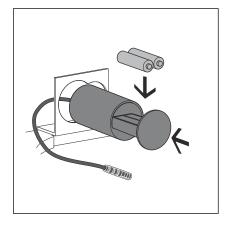
Insert new battery and close battery compartment.
