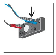
Connect the black cable of the power supply to the outer right connection of the control.
