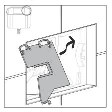
Lead the panel into the cistern at an angle.
