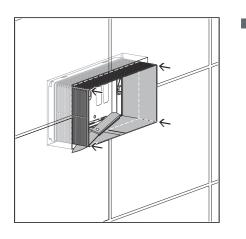
Cut the corners of the revision shaft vertically through to the wall surface.
