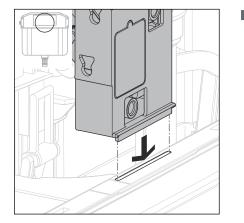
Insert the mechanism. The mechanism must sit exactly in the recesses of the cistern.
