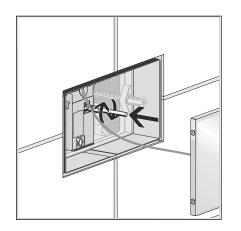
Screw actuating rod into the top right of the mechanism. If necessary, shorten the actuating rod.
