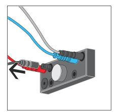
Remove the cable of the programming contact.
