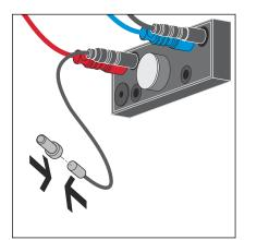
Hold the magnetic pin in front of the programming contact.
