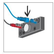
Connect the blue connection cable from the sensor to the blue connection of the control.
