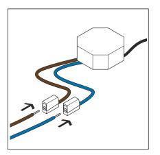
Push the connection cable into the terminals.
