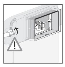
Close the corner valve to shut the water supply off.
