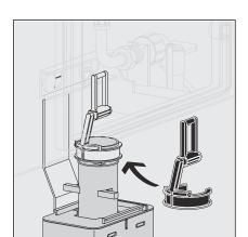
Push the bow onto the drain valve from the left.
