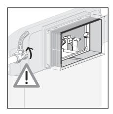
Open the corner valve to enable the water supply.
