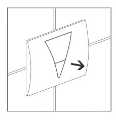
Loosen the support at the top and the bottom and remove it from the installation shaft straight forward.
