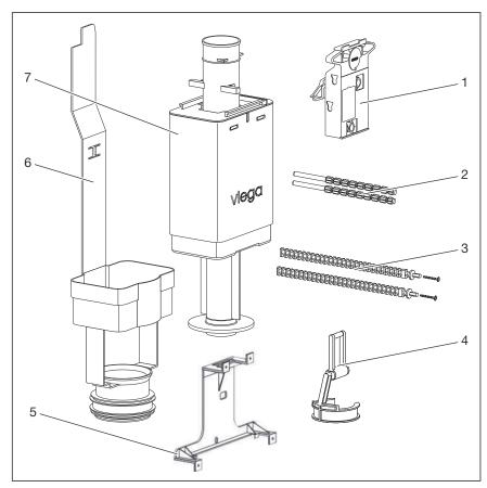
Fig. 1: Drain valve set
