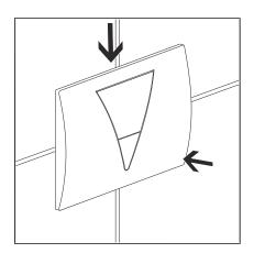
■ Hang the flush plate from above in the basic panel press in below.
