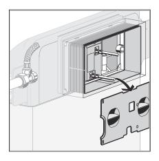
Remove the cover straight forward from the installation shaft.
