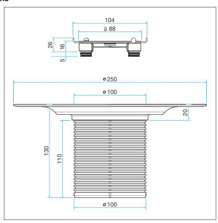
Fig. 2: Installation dimensions
