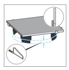
If necessary, cut the tiled grate to tile-level.
