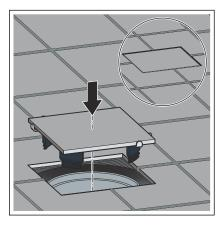
Fit the tiled grate into the stacking element or into the drain unit.
