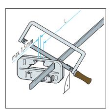
**NOTICE!** The standing grate must not be shortened with a cutting disc (angle grinder).
