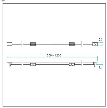
Fig. 2: Installation dimensions
