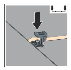
Place the standing grate holder on the adjusting screw and adjust to tile level.
