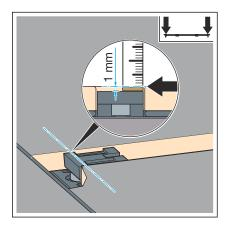
The upper edge of the standing grate holder must be approx. 1 mm below the upper edge of the tiles.
