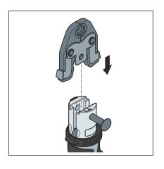
Insert the press jaw in the press jaw fixture of the cylinder head.
