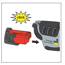
Insert the battery into the device as illustrated until the battery engages.
