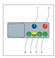
Fig. 4: Start button with status LEDs
