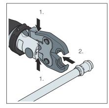
After full retraction of the roller head, open the press jaw and loosen it from the press connector.
