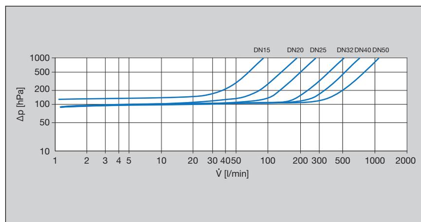
Fig. 2: Performance diagram pressure loss CRV press/threaded connection
