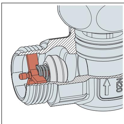
The cone seal is pre-stressed with a spring and is held in position by a soldered strut. The spring slackens and pushes the valve cone into the outlet. The gas flow is then blocked and the valve is now permanently closed gas-tight.
