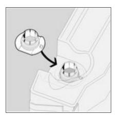
Push wall lead-in from inside into the upper opening.
