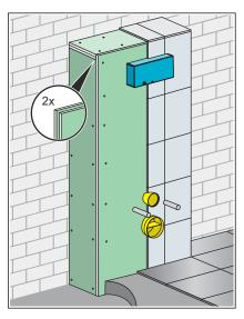
Double-clad WC element with IFGP cladding panels (model 8055.10) (2 x 12.5 mm).
