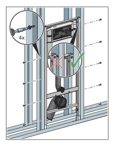
Attach WC element to the support profiles using the screws supplied.
