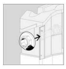
Pull the corner valve inwards out of the wall lead-in.
