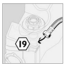
■ Re-mount (SW 19) the flexible hose onto the corner valve.
