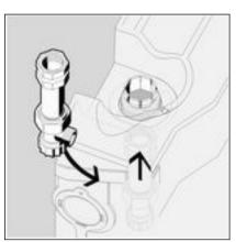
Insert the corner valve back into the wall lead-in.
