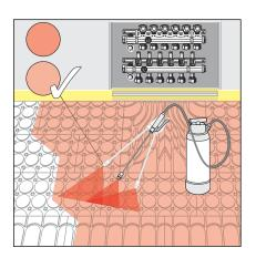
Applying the casting compound
