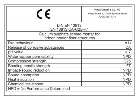
Fig. 1: Fonterra Reno casting compound, CE mark
