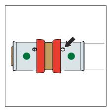
Check the position of the seal ring and the insertion depth of the pipe in the press collar before pressing.
