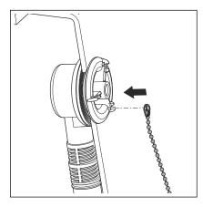
Hang the free eyelet of the chain onto the bottom hook of the fixing flange.
