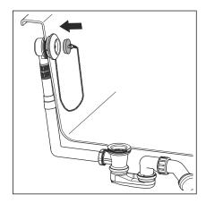
The valve plug can be inserted into the rosette for safe-keeping.
