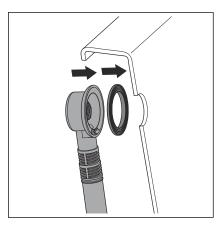
Fit profile seal in the overflow unit.
