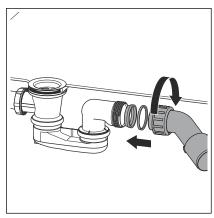
Align the odour trap in such a way that the drain elbow can be connected to the wastewater pipe.
