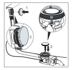
To avoid damage to the rosette and valve cone, mount the equipment set only after finishing all other work on the building site. Proceed as follows:
