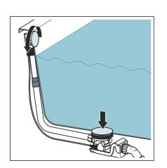
The drain / overflow are controlled via the rotatable rosette on the overflow. Proceed as follows to open or close the drain:
