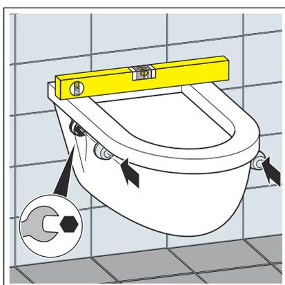
► Align the WC ceramic and re-tighten fixing screws.
