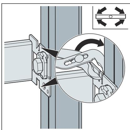
► Bend the sides of the metal bars of the rails.
