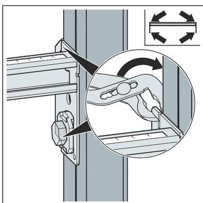
► Bend the sides of the metal bars of the fitting holder.
