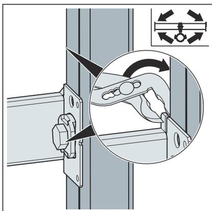
► Bend the sides of the metal bars of the drain elbow.
