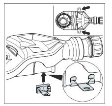
Attach the retaining clamps.
