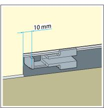
Push the standing grate holders at both sides of the shower channel to a position at 10 mm distance from the tile covering.
