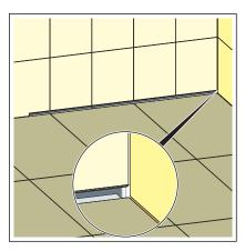
Use the mounting adhesive supplied to close the gap in the corner area.
