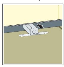
**NOTICE!** Risk of damage during cleaning! To protect the shower channel and the tiles, use the tile protection and checking tool comprised in the delivery.
