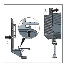
Position the foot and push the profile into place. The foot can be moved on the base unit.
