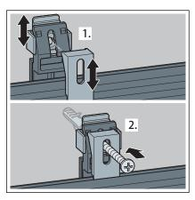
■ Use the spacer (1) to adjust the shower channel to the wall situation.
