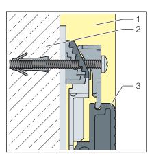
Fig. 19: Wall with 25 mm plaster layer
