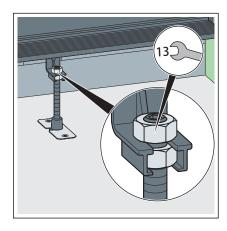
Fix the foot height adjustment with lock nuts.
