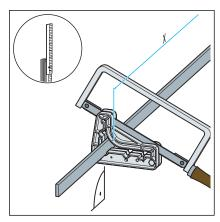
If required, shorten the standing grate with a handsaw and deburr.Do not use a circular saw or angle grinder.
