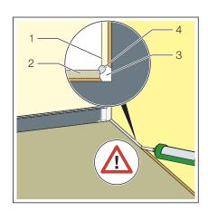
■ Use suitable filling material to close the gap in the corner area.
