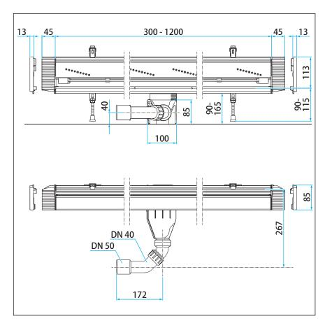
Fig. 18: Dimensions of base unit basic model
