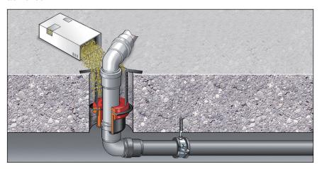
Fig. 16: Example: fire protection pipe lead-in
