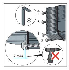
Screw the closing piece onto the profile straight until approx. the last 2 mm.
