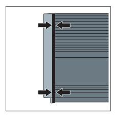
When mounting on an uninterrupted wall □ The closing cap is properly mounted when the seal is pushed together gently.
