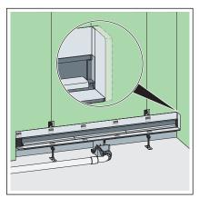
Embed the shower channel into the gypsum plaster board wall.
