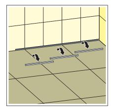
Optionally, a sieve can be inserted. When using the sieve, the drainage capacity drops by 0.05 l/s per drain.
