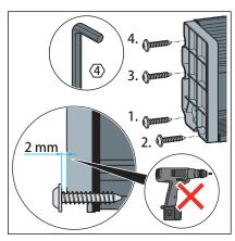
Screw the closing cap onto the profile straight until approx. the last
