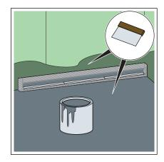
Apply the first layer of bonded sealing generously onto the screed and the wall.
