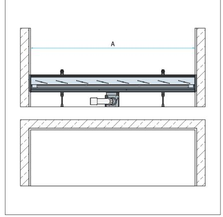
Fig. 2: Shower channel in the niche: masonry walls on left and right sides
