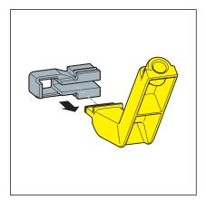
Push the standing grate holder (part A) on the mounting tool.
