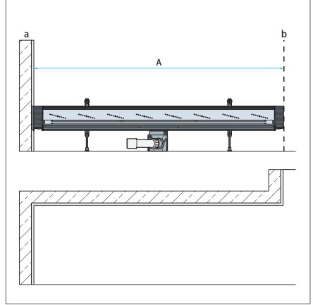
Fig. 8: Shower channel in the corner: masonry wall on left, glass partition on right, internal closing pieces left and right side
