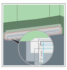
Place the sealing tape strips on the flange in such a way that flange and screed are evenly covered.
