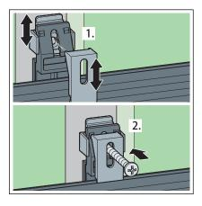
■ Use the spacer (1) to adjust the shower channel to the wall situation.
