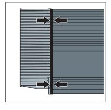
□ The closing piece is properly mounted when the seal is pushed together gently.
