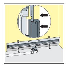
Embed the shower channel into the plaster or into the rigid foam board.
