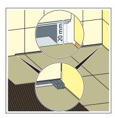
**INFO!** The gap for the standing grate must be exactly 20 mm. Use the tile protection tool and control tool to define the gap size.
