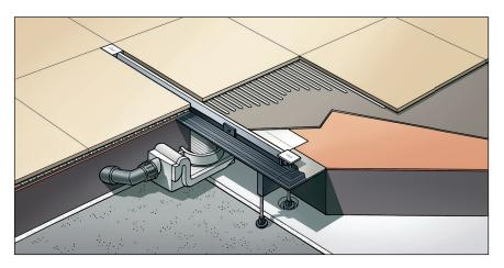
Fig. 14: Diagram of a bonded seal
