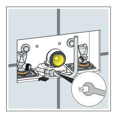
Manufacture the connection for the washbasin fitting on one side using the copper pipe supplied.
