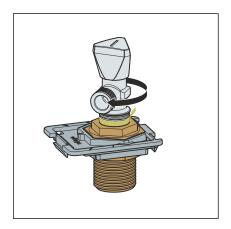
Screw the corner valve into the screw fitting.
