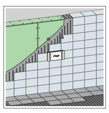
Clad the element with suitable plasterboard cladding panels.
