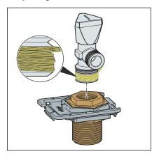
Seal the corner valve (e.g. using hemp).
