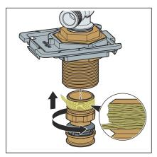
Seal and screw in a suitable pipeline adapter.
