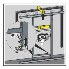
Set the height of the element by means of the feet.
