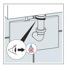
Turn the drain elbow to the right and in doing so secure it to the washbasin.
