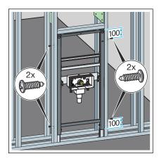
Attach the element to the stud frame using the screws supplied.
