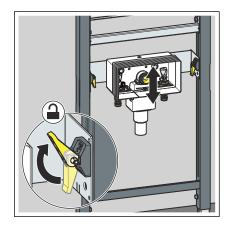
Use the quick release to adjust the drain elbow to the desired height.
