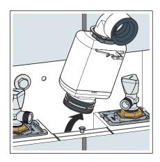
Remove the odour trap for cleaning.
