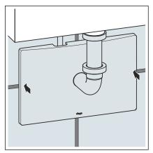
Attach the cover plate to the concealed connection box.
