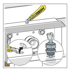
**INFO!** Optional cable bushing On the top of the concealed connection box a section can be cut out which, for example, can be used as a cable passage.
