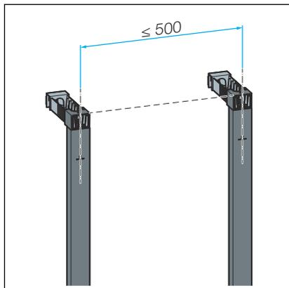
Fig. 3: Maximum interval between Prevista Dry support brackets
