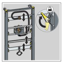
Use the quick releases to adjust the ledges for drain elbows, supply fittings and urinal fixing to the desired height.
