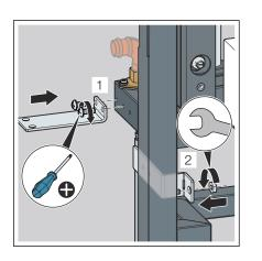
Mount retaining plates 1 and 2. They can be attached on the left and right hand side of the element.
