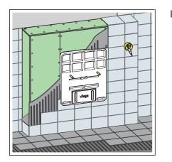
Tile up to the mounting template and concealed socket.
