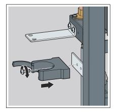
Mount the pipe clamp for the waste elbow to retaining plate 2.
