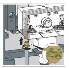
Seal in the flexible hose on the thread side and assemble on the wall lead-in of the concealed connection box.
