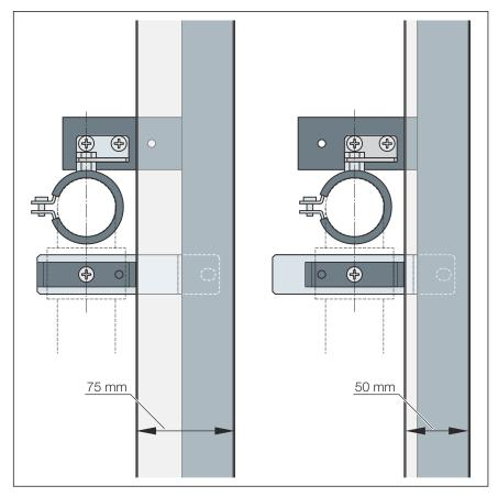
Fig. 2: Minimum distance to the wall
