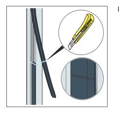
▶ If necessary, cut the seal to the appropriate length.
