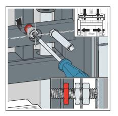
Tighten the rear threaded nuts at all four points (SW 17). When doing so, hold the threaded bolts with a flat-blade screwdriver.
