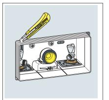
Cut the concealed connection box flush with the cover plate INFO! Take care when cutting! Do not damage the cover
