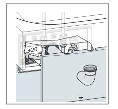
Attach the cover plate to the concealed connection box. The lateral supports serve as a safeguard against distortion.
