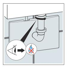
Turn the drain elbow to the right and in doing so secure it to the washbasin.
