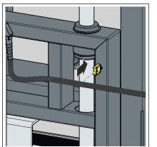
Re-mount the hydraulic hose in the guide provided on the rear side of the washbasin element.
