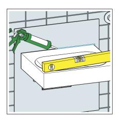
Fasten the washbasin and seal using silicone.
