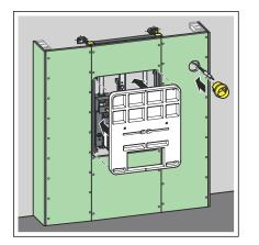
Install the concealed socket and mounting template.
