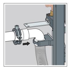
Make the wastewater connection (DN 40) on site.
