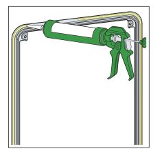
Apply the silicone seal to the rear of the cover frame.
