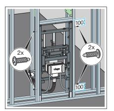
Attach the element to the stud frame using the screws supplied.
