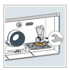
If the corner valve has to be replaced, proceed as follows:
