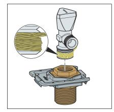
Seal the corner valve (e.g. using hemp).
