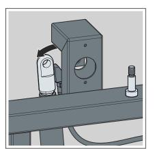
Swing out the gas pressure spring to the left or right-hand side.
