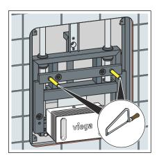
Shorten the threaded bolts for fixing the sanitary ware according to the ceramic used.
