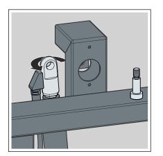
Turn the head of the gas pressure spring with the hydraulic hose by 180°.
