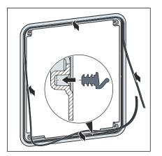
Fit the supplied seal in the cover frame on the front.
