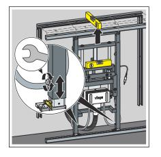
Set the height of the element by means of the feet.
