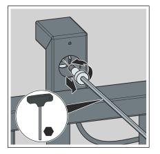
Undo the Allen screw (size 5) on the head of the gas pressure spring.
