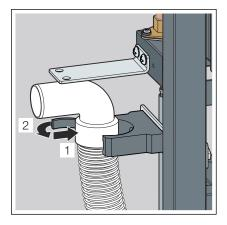
Mount the waste elbow in the pipe clamp.
