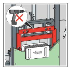
The plasterboard cladding panels must not be screwed together with the height-adjustable internal frame!
