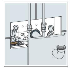
Set the odour trap to the right size at the height. The vertical setting range is 20 mm.
