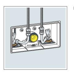
Optionally, connect the washbasin fitting to the concealed connection box using flexible hoses.
