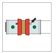
Check the position of the seal ring and the insertion depth of the pipe in the press collar before pressing.
