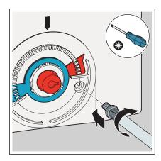
Screw the upper part of the housing to the casing base.
