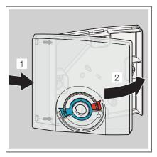
■ To close the housing, hook the upper part of the housing on to the left side of the housing and then press it down on the right until it audibly clicks into place.
