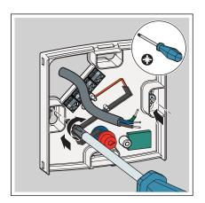
Fasten the casing base to the wall (non-conductive substrate) or to a concealed socket.
