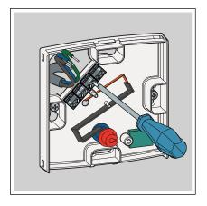
Connect the cables in accordance with the connection plan, see ∜ 'Connection diagram' on page 8.
