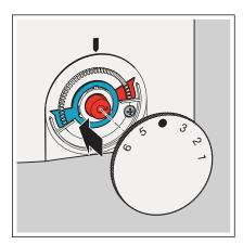
**NOTICE!** Do not place the rotary knob on the room thermostat until the upper part of the housing has been fitted.
