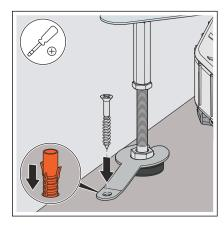
Secure the feet in place with the fixing material.
