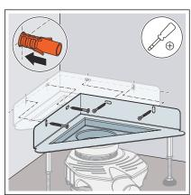
**INFO!** In the case of even wall surfaces in combination with thin layers of adhesive, the installation depth of the wall sheet has to be agreed with the tiler. If necessary, the wall sheet will have to be embedded into the wall.
