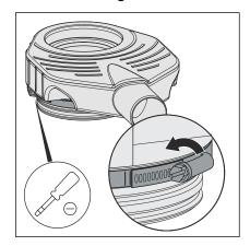
Loosen the fastening ring with a screwdriver.
