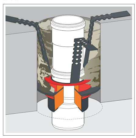
Fig. 3: Example: fire protection pipe lead-in
