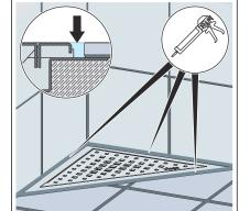
Seal the joint between the grate frame and the tiles with silicone.
