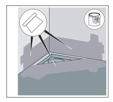
Apply the second layer of bonded sealing generously onto the sealing tape, screed and wall.
