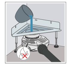
The drain must now be lined with screed and sealed & Chapter 3.2.6 'Sealing the corner drain' on page 25.
