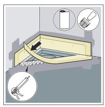
Position the sealing tape on the flange so that the flange and screed are uniformly covered.
