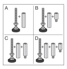
Depending on the desired installation height, additional height adjustments may have to be mounted in addition to the feet:
