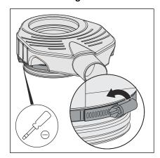
Loosen the fastening ring with a screwdriver.
