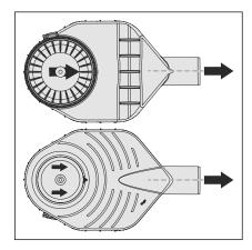
The arrow on the base of the odour trap must be pointed towards the drain.
