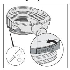
Loosen the fastening ring with a screwdriver.
