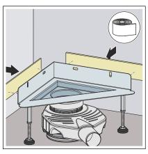
Attach the sound protection strip on the wall side of the sealing flange.
