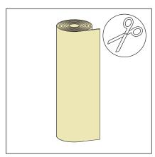
Cut the sealing tape generously. The strips should overlap when stuck on.
