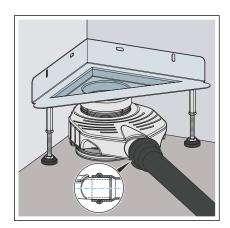
Push the drain socket into the drainpipe completely.
