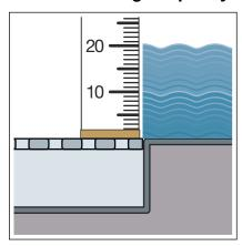
The drainage capacity is dependent on the chosen installation height. The installation height is the distance from the drain to the flange.
