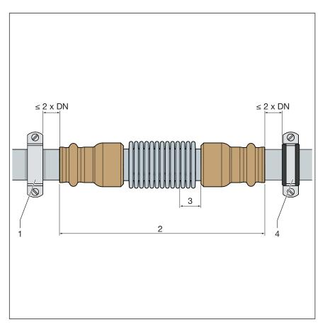
Fig. 1: Compensator installation information
