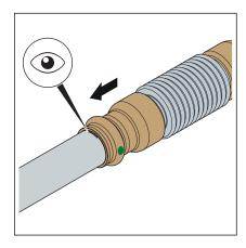
Push the compensator all the way on.
