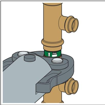
► Press the two T-pieces, incl. press-in nozzle.
