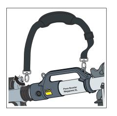
Use clasps to fasten the strap ends to the Press Booster and the press machine.
