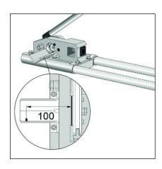
□ The tolerance range for the rail length is 10 mm. The stability is not compromised.
