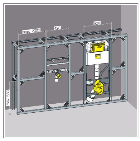
Fig. 19: Interval between vertical rails
