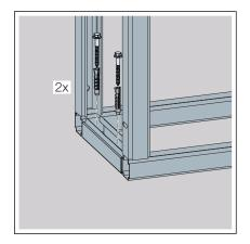
With free-standing pre-wall constructions, all floor rails must be fastened to the floor using the fixing material supplied. Even the short rails must be fastened using at least two screws.
