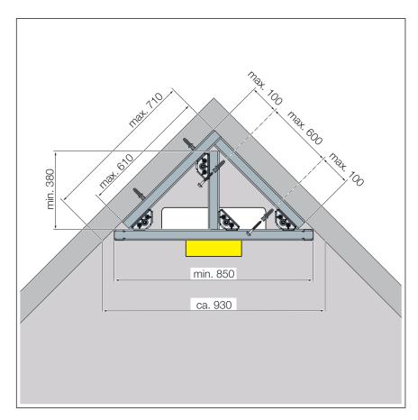
Fig. 8: Installation dimensions corner mounting
