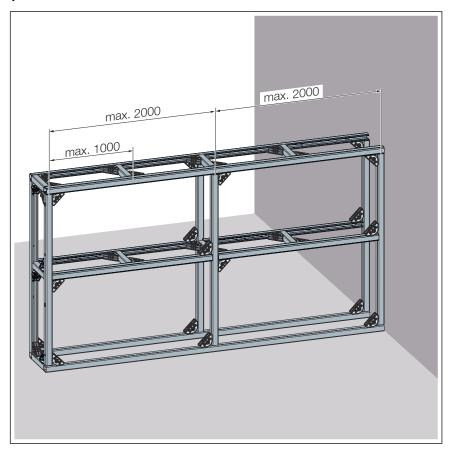
Fig. 9: Installation dimensions half-height room partition (one-sided connected)
