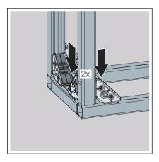
Stabilise each corner of the floor rails using two rail connectors.
