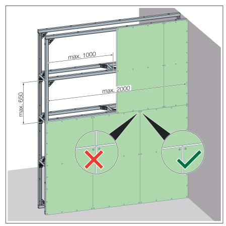
Fig. 14: Installation dimensions partition and room-height room partition
