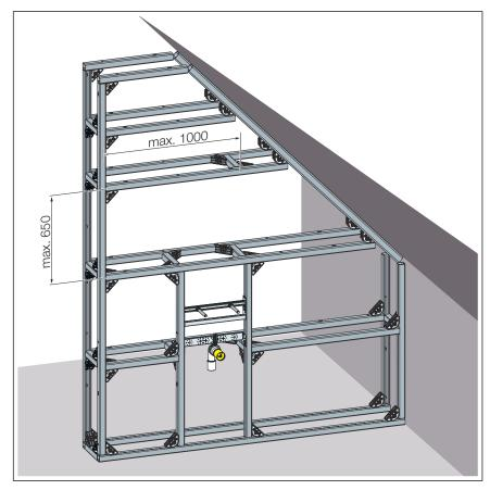
Fig. 16: Installation dimensions partition on the roof slope
