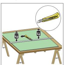
■ Use a plasterboard blade to cut into the cardboard at the front.
