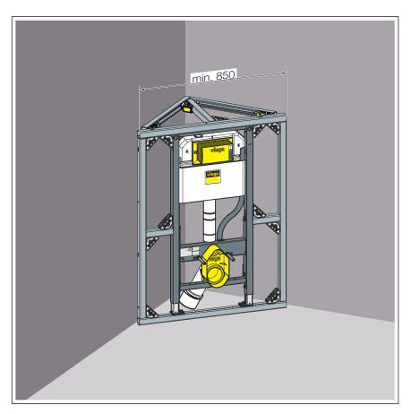
Fig. 7: Installation dimensions corner mounting
