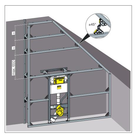
Fig. 15: Installation dimensions pre-wall on the roof slope
