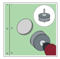
Make the pipe penetrations with a hollow wall box cutter, or with a jigsaw for larger diameters.
