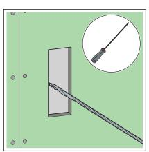
■ Cut out the installation recesses with a jigsaw or an electric jigsaw.
