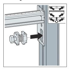
Secure the module onto the open mounting rail with the slot nuts. Insert the slot nut into the opening of the module.
