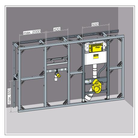
Fig. 3: Installation dimensions half-height pre-wall
