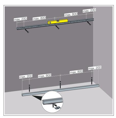
Fig. 31: Rail fixing dimensions
