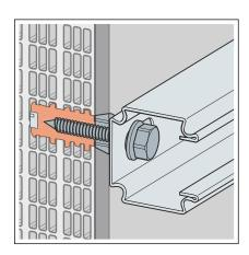
Fig. 30: Injection mesh anchor
