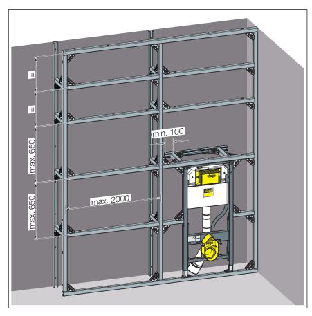
Fig. 4: Installation dimensions room-height pre-wall
