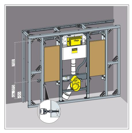
Fig. 6: Barrier-free mounting, version 2
