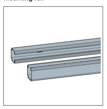
The mounting rail made of galvanised steel is 5 m long, open on one side and perforated every 30 cm for wall and floor mounting.
