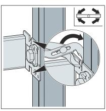
■ Bend the sides of the metal bars of the rails.
