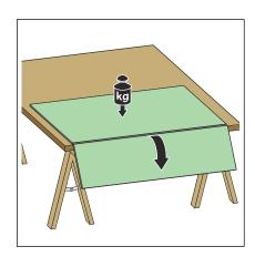
■ Break the plasterboard in the cut.
