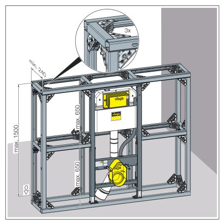
Fig. 11: Installation dimensions half-height room partition (free-standing)
