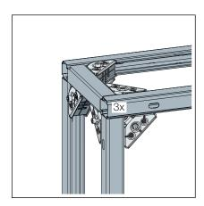
Fig. 22: Rail connector top
