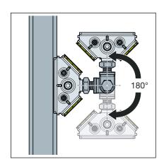
Connections with an angle of up to 180° can be made using the joint.
