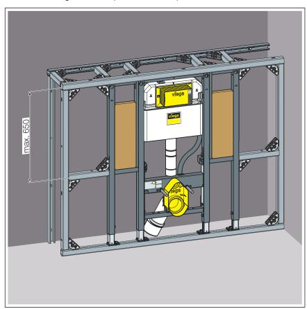
Fig. 5: Barrier-free mounting, version 1
