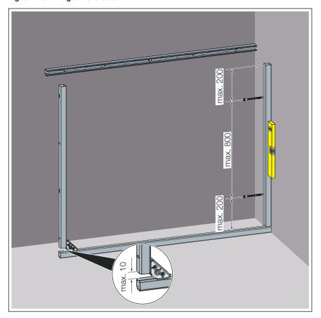
Fig. 32: Rail fixing dimensions
