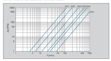
Fig. 1: Performance diagram slanted seat valve press/threaded connection
