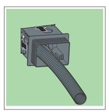
Insert the concealed socket into the gypsum cladding panel.
