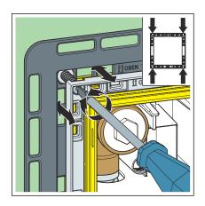
Set the installation frame to the measured depth.
