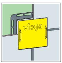
$\hfill \hfill \supset$  The installation frame has been mounted and the flush plate can be mounted.
