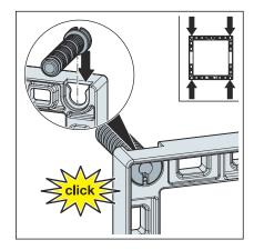
Insert the bolts in the installation frame.
