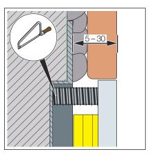
■ Measure the distance from the cladding to the tile level.
