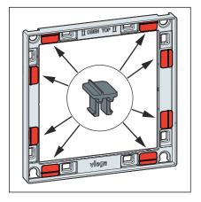
Insert the clips into the installation frame for the urinal flush plate Visign for More 200 glass / wood.
