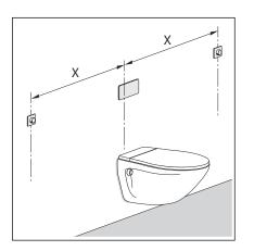
The corresponding empty pipe (included in the scope of delivery of the remote actuation) is required when preparing the remote actuation Visign for Public1 (model 8326.21).
