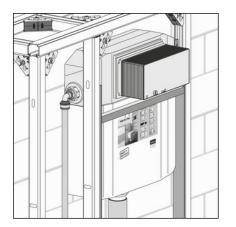
Install site protection of the flush actuation.
