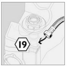
Re-mount (SW 19) the flexible hose onto the corner valve.
