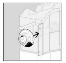
Pull the corner valve inwards out of the wall lead-in.
