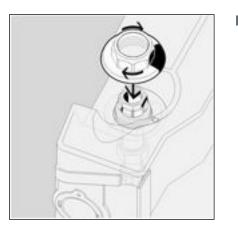
Screw plastic union nut back onto wall lead-in.
