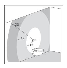
Lead empty pipe from the switch or button into the concealed cistern, to connect the concealed socket and concealed cistern.
