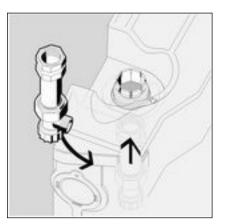
Insert the corner valve back into the wall lead-in.
