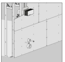
Single clad pre-wall: Clad with 12.5 mm wide IFGP or 12 mm wide Aqua-KS cladding panels.
