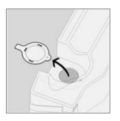
Loosen the closing cap on the left-hand upper side of the concealed cistern.
