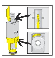
The WC module is factory-set at a small flush volume of approx. 3 I. The small flush volume can be set at three levels: approx. 3 | / 3.5 | / 4 |.
