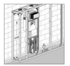
Align the height of the module in accordance with the cutting check. Whilst doing so, observe the markings on the cistern. The height is 1000 mm above UEFFL.
