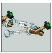
Tighten the lock nuts of the water meter screw connection.
