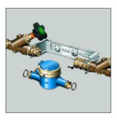
Loosen the fixing nut of the slide and push in the slide.
