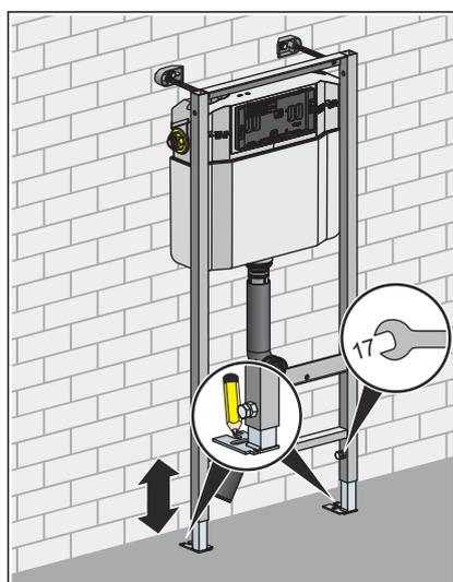
► Align the height of the feet with a fork spanner (size 17).
