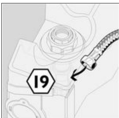
► Re-mount (SW 19) the flexible hose onto the corner valve.
