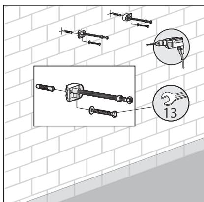
► Attach fixing set with the fork spanner (size 13).
