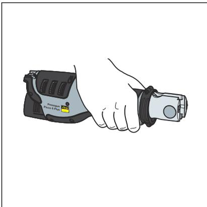
➤ To prevent injury during the pressing, hold the press machine at the gripping surface provided as shown.
